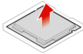
Figure 113. Pivoting the microprocessor socket upward
